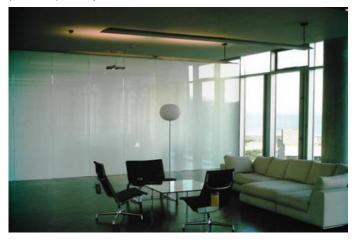
When the power is switched off the liquid crystal molecules are randomly oriented scattering light and the switchable Smart Film becomes opaque.
